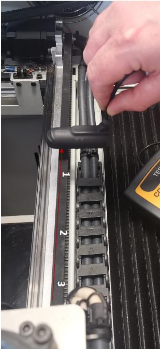
Fig. 45 Measurement location of the timing belt tension on the Y axis
