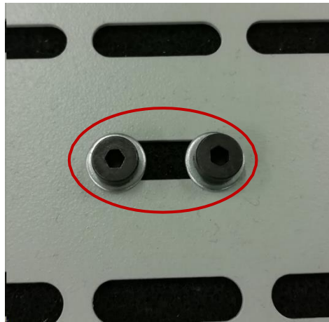
Fig. 11 Unscrewing 6 DIN7984-M4x6 screws from the top cover of the printer
