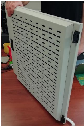
Fig. 17 Placing the top cover
